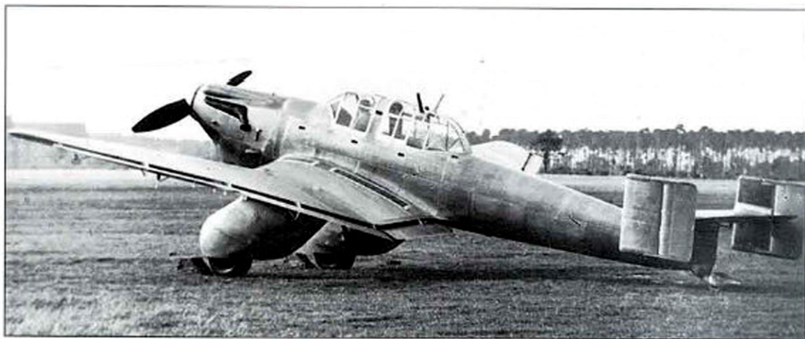
The first prototype Junkers Ju 87 V1 featured a twin-tail unit, but during a medium-angle test dive this assembly began to oscillate. When the pilot attempted to recover, the entire starboard vertical surface parted company with the rest of the tail section, causing the aircraft to crash
