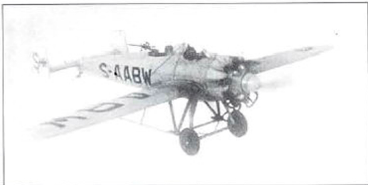
Equipped with a 480 hp Bristol Jupiter VII engine, the first prototype Junkers K 47 is here seen bearing its initial Swedish civil registration, S-AABW. After subsequent evaluation at Lipetsk, this machine – re-engined with the 540 hp Siemens Sh 20 – was assigned to the DVL (German Aviation Experimental Establishment) at Berlin-Adlersdorf as the Junkers A 48 dy, registration D-2012
