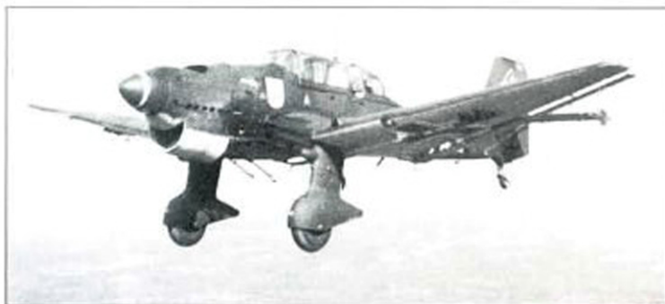
A Ju 87B-1 of StG 77 returns from a sortie with its underwing bomb-racks empty and the bomb cradle fork swinging freely in the slipstream. Note that this aircraft also appears to have a name written ahead of the Staffel badge – a not uncommon practice among Stuka units
